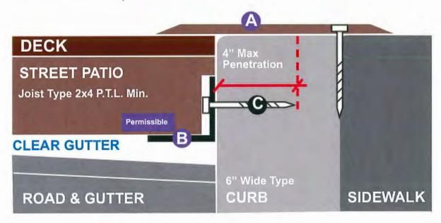
The top of the Street Patio platform must be flush with the sidewalk with a maximum gap of 1/2 inch between the curb and the top of the deck.
