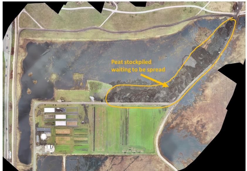
Peat windrows piled at the edge of the north field expansion area waiting to be spread across the north field. Feb. 2023
