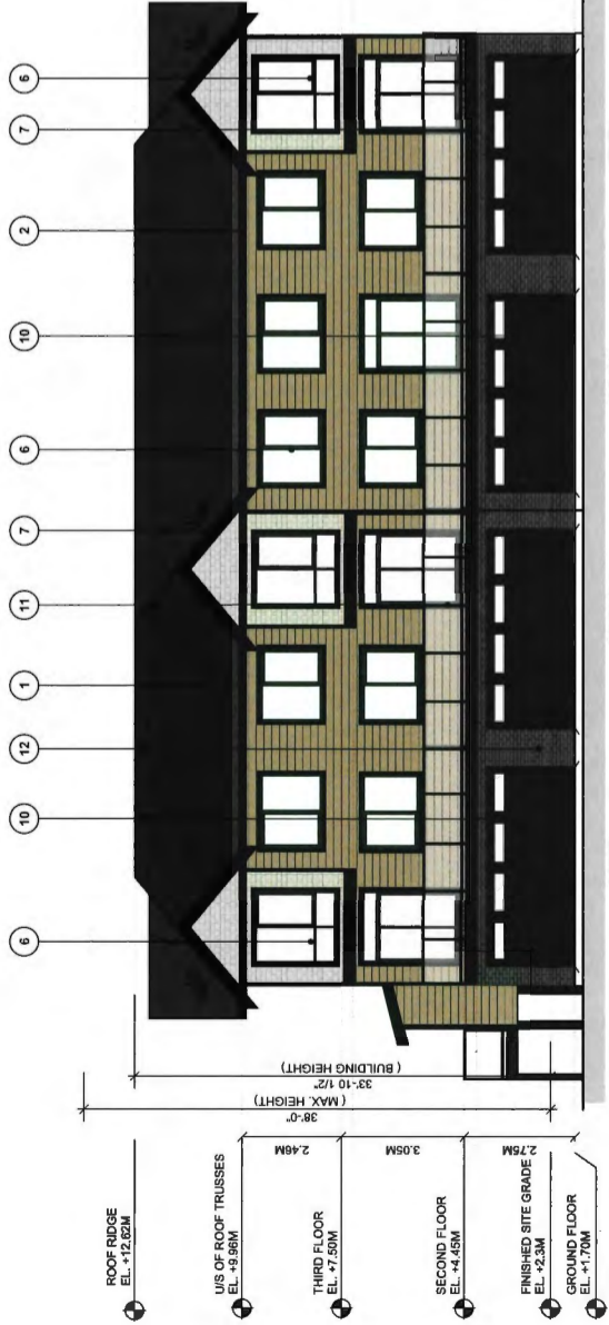
BLDG. 11: NORTH ELEVATION -SCHEME D
