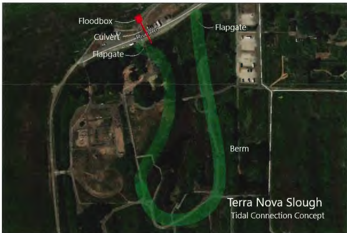
Figure 7: Option 3 – Tide Gate and Flood Berm
