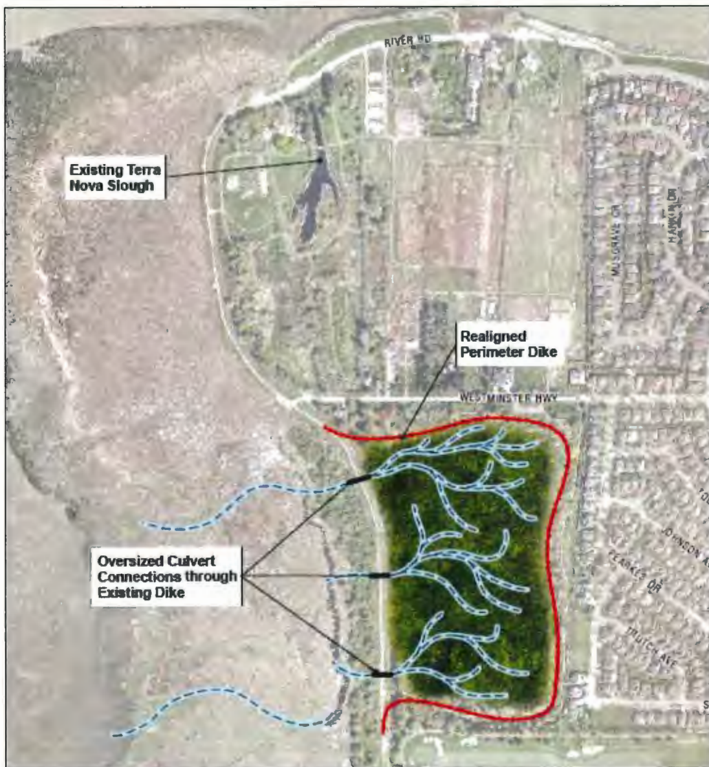
Figure 11: Option 5 – Connect and Enhance Existing Wetlands in Terra Nova Nature Area
