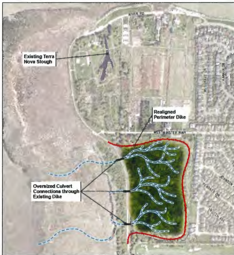
Figure 4: Option 5 - Connect and Enhance Existing Wetlands in Terra Nova Nature Area
