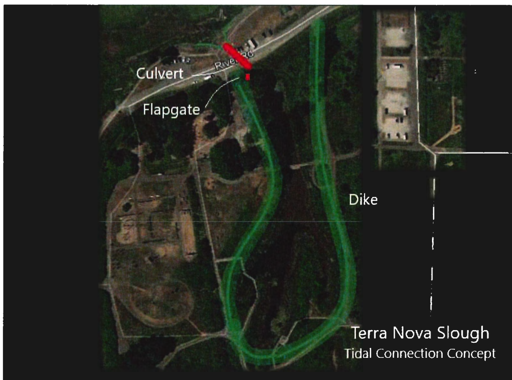
Figure 6: Option 2 – Open Culvert and Ring Dike
