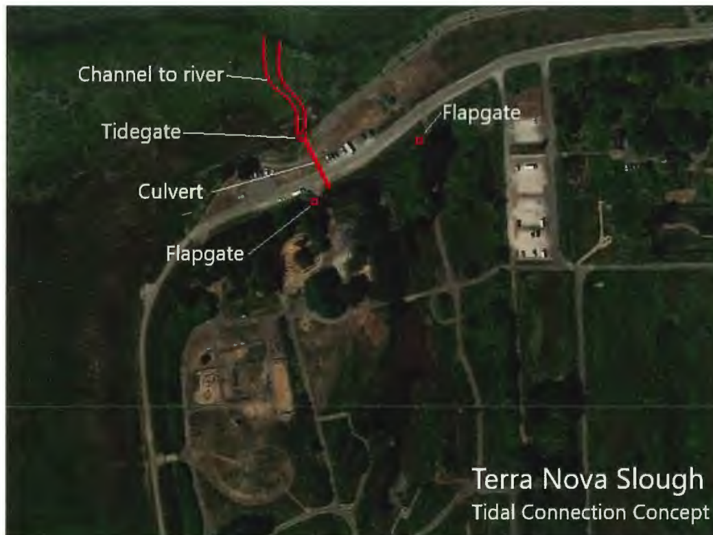
Figure 4: Option 1 – Floodbox with Self-Regulating Tide Gate
