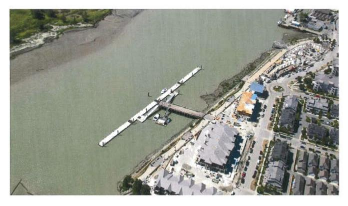
(Option 1) New 600'-0 Breakwater Floating Dock (example photo shown below)
