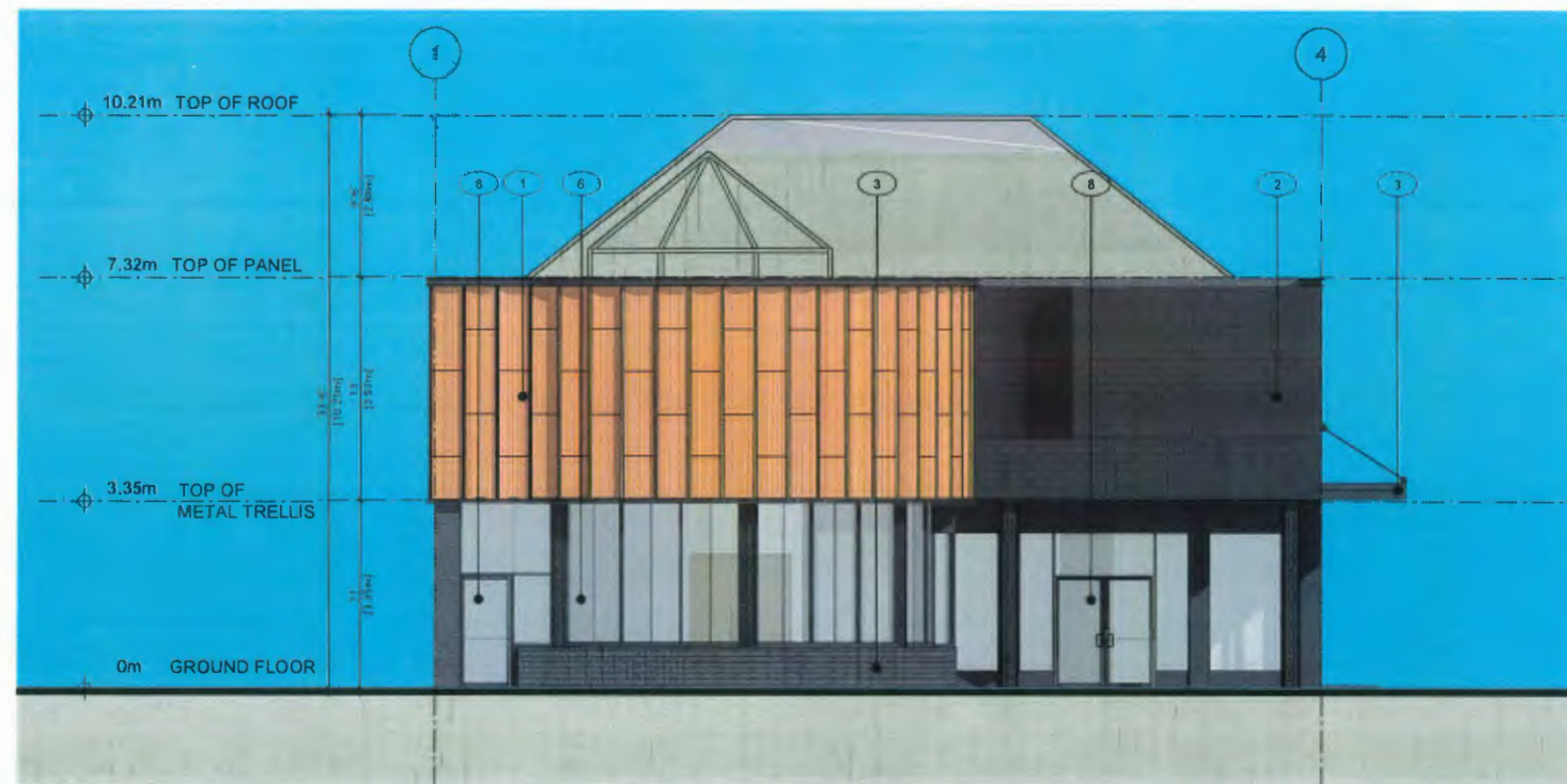
2 PROPOSED BUILDING ELEVATION-SOUTH Scale: 3/16"=1'-0"
