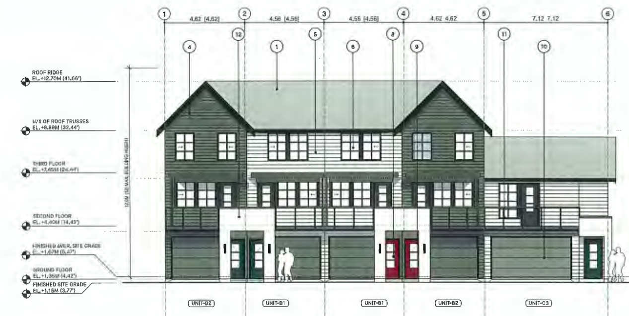
SOUTH ELEVATION - DRIVE AISLE
