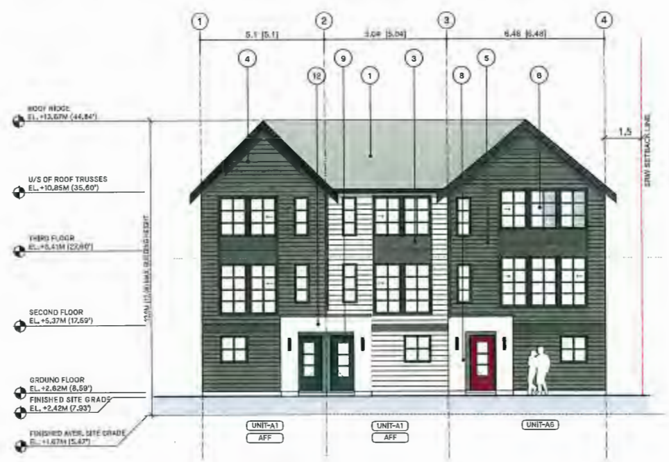
WEST ELEVATION - NO1 ROAD
