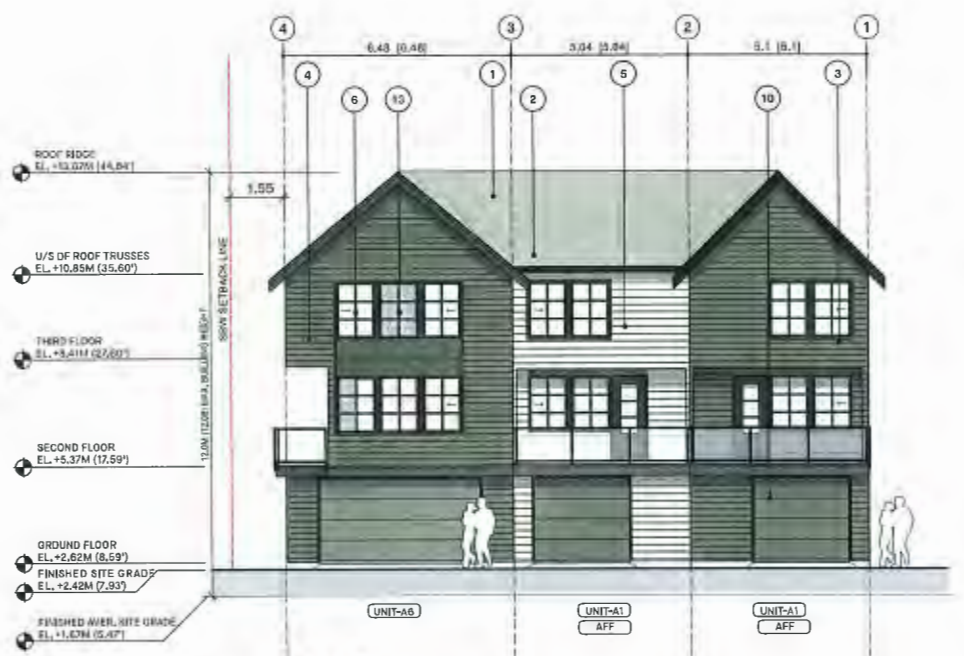
EAST ELEVATION - DRIVE AISLE
