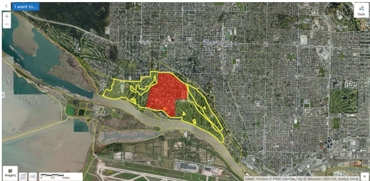
FIGURE A6. LADNER SOIL SERIES MAPPED LOCATIONS - OUTLINED IN SOLID YELLOW. LOCATIONS HIGHLIGHTED IN RED REPRESENT THE MOST IDEAL AREA(S) FOR SOURCING OF THIS PARTICULAR SOIL ASSOCIATION.
