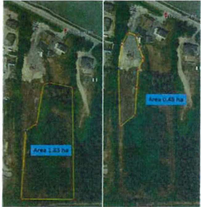
Figure 21. Area measurements at 21700 Riverside Rd delineating the area already filled, and the area requiring fill (from Google Pro)
