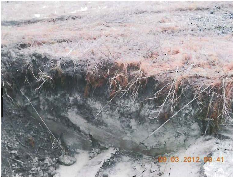
Photograph 8 Typical Delta Soil Profile identified on the NW portion of the Site.
