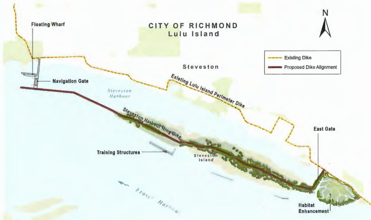
Figure 1. Steveston Island Dike Layout
