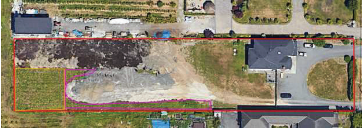
Figure 8 Fill areas requiring alteration (grading and/or more fill)
