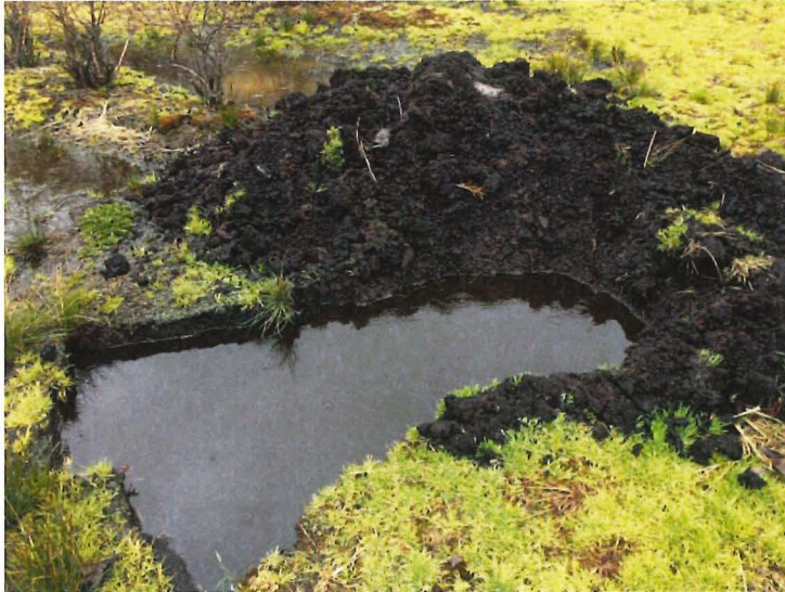
PHOTO 9. SOIL PIT EXCAVATED NEAR PIT 3 IN THE PREVIOUS WEEK THAT FILLED WITH WATER AND HAD TO BE ABANDONED.
