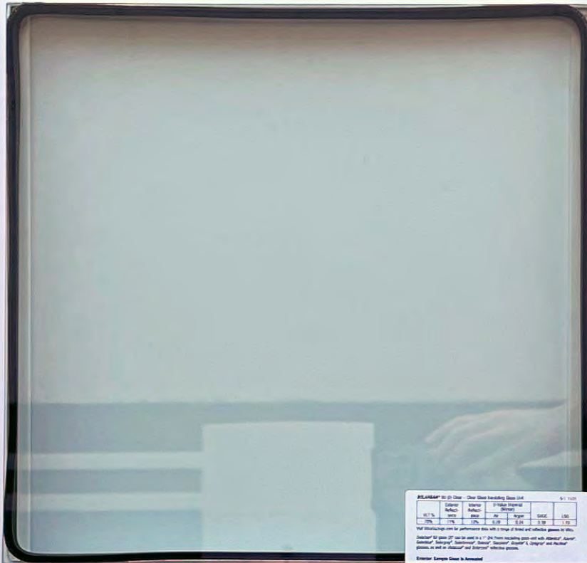
Solar Control Low-E Double Insulated Glazing - Door & Operable Window Solarban 60*8mm + Air 12.7mm + Clear 6mm
