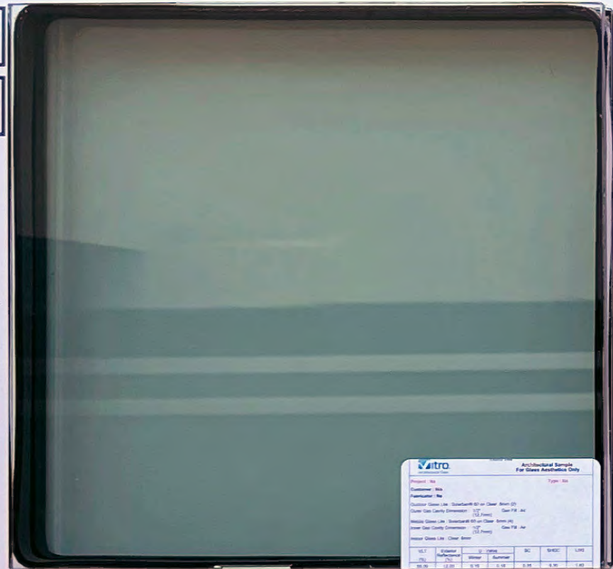
Solar Control Low-E Triple Insulated Glazing Unit Solarban 60*8mm + Air 12.7mm + Clear 6mm + Air 12.7mm + Solarban 60*6mm
