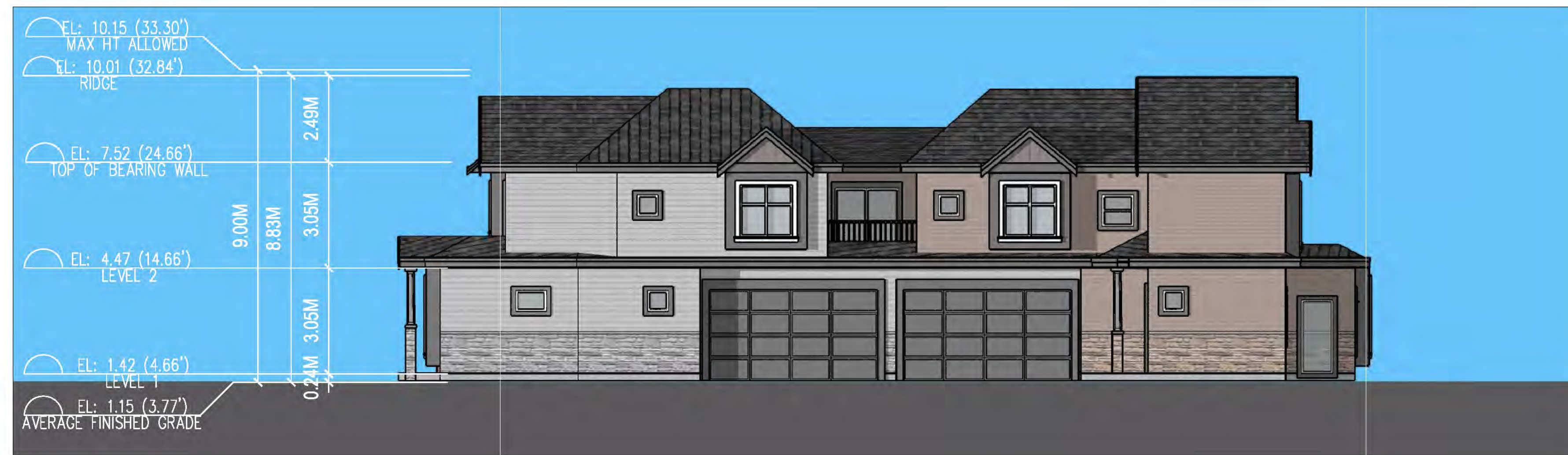
3 BUILDING A EAST ELEVATION A3.1 SCALE: 1/8"=1'-0"
