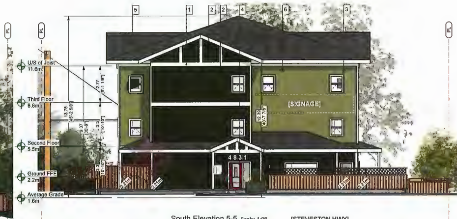
South Elevation 5-5 Scale: 1:96 [STEVESTON HWY]
