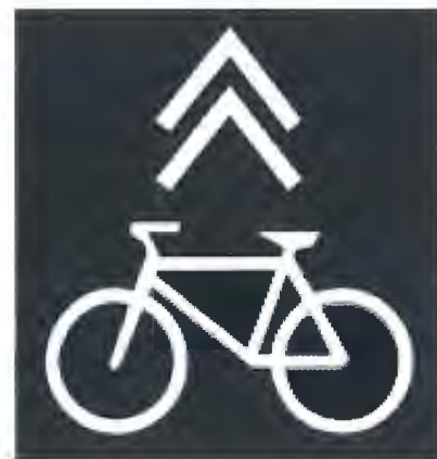
"Sharrow" Pavement Marking
