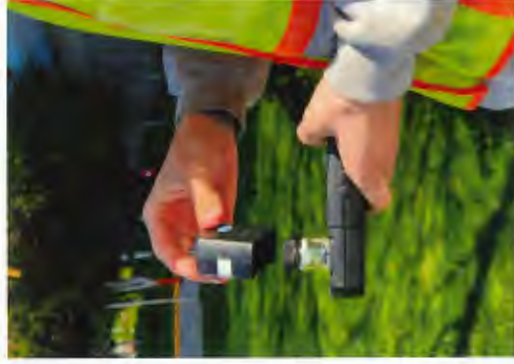
Checking the chlorine residual of a water sample using a chlorometer.
