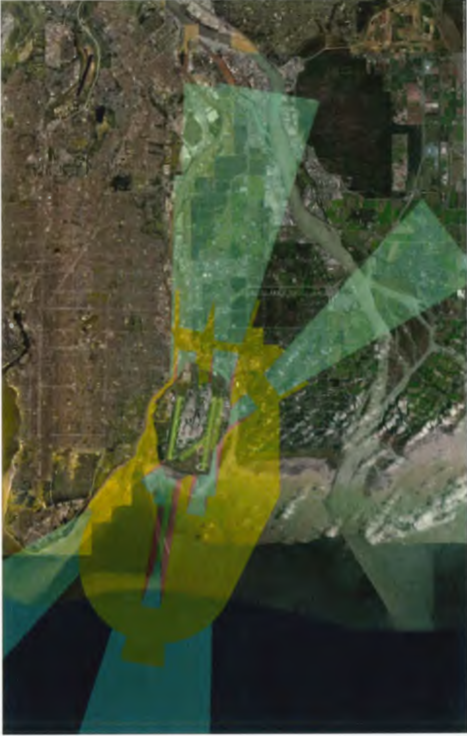
Yellow Colour: Outer surface (45m building height limit above ground) Teal Colour: Take-off/approach surface (variable height limit) Red Colour: Transitional surface (variable height limit)
