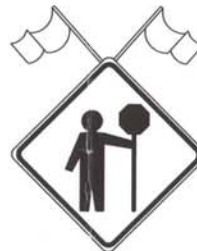
TRAFFIC CONTROL PERSON AHEAD (C-28) - 75x75 - Black on Orange - with flags (High Level Warning Device) - QUANTITY :1
