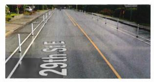
Figure 1: Example of Buffered Bike Lane with Delineator Posts (29th St E, North Vancouver)
