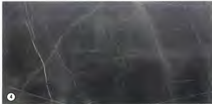
4 DARK GREY STONE TILE FEATURE RECESSED CLADDING AT ENTRIES & AMENITIES MARBLE TILE 'PIETRA GRAY' (or SIM. CREO STONE)
