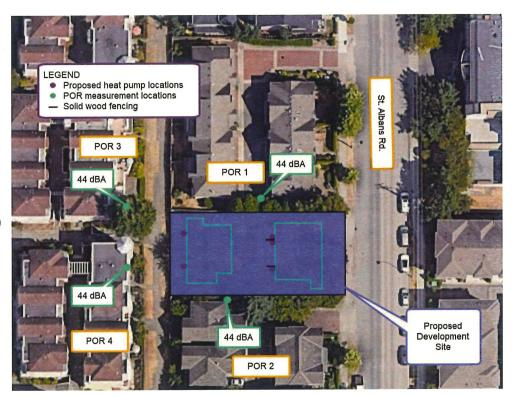
Figure 2: Aerial photograph showing bylaw PORs and predicted heat pump noise levels.
