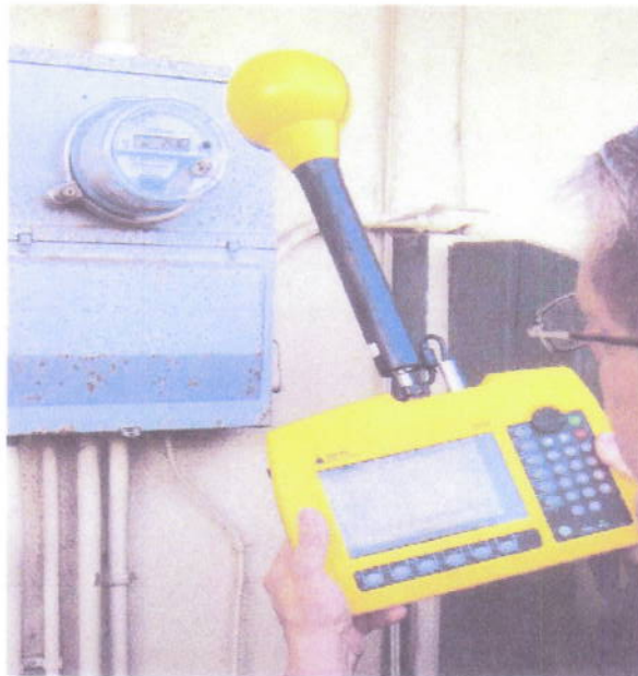
Figure 1 - Technician Measuring the RF power density from a Smart Meter
