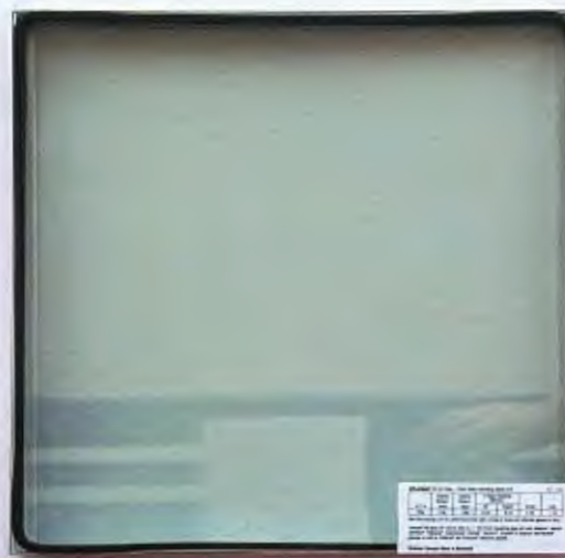
Solar Control Low-E Double Insulated Glazing - Door & Operable Window Solarban 60'8mm + Air 12.7mm + Clear 6mm
