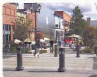
Pedestrian priority over vehicles reinforced by: pavement changes, pedestrian scale lighting, wide sidewalks and landscaped seating areas reinforce pedestrian priority over vehicles, overall character and street activity.
