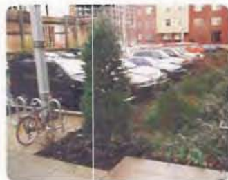
Permeable landscaped strip-walk collects run-off water from the paved parking lot allowing natural absorption of rain water and contribute to irrigation.
