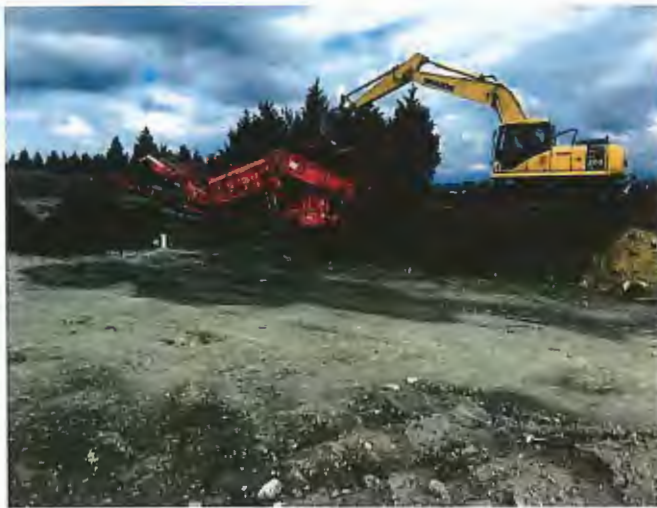
Photograph 16: Soil reclaimer intended for use to screen soil and produce sand loam for filling purposes
