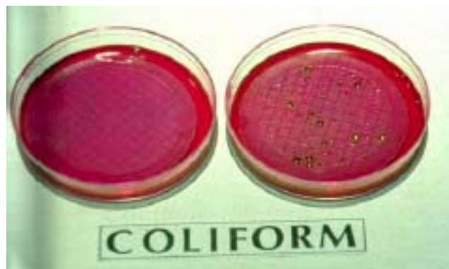
Figure 4b: Laboratory Test Sample Clear Coliform Detected
