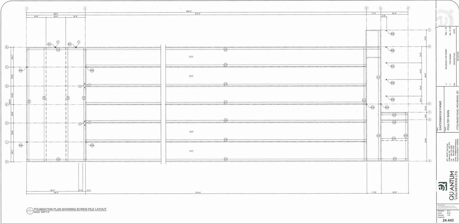
1 FOUNDATION PLAN SHOWING SCREW PILE LAYOUT
