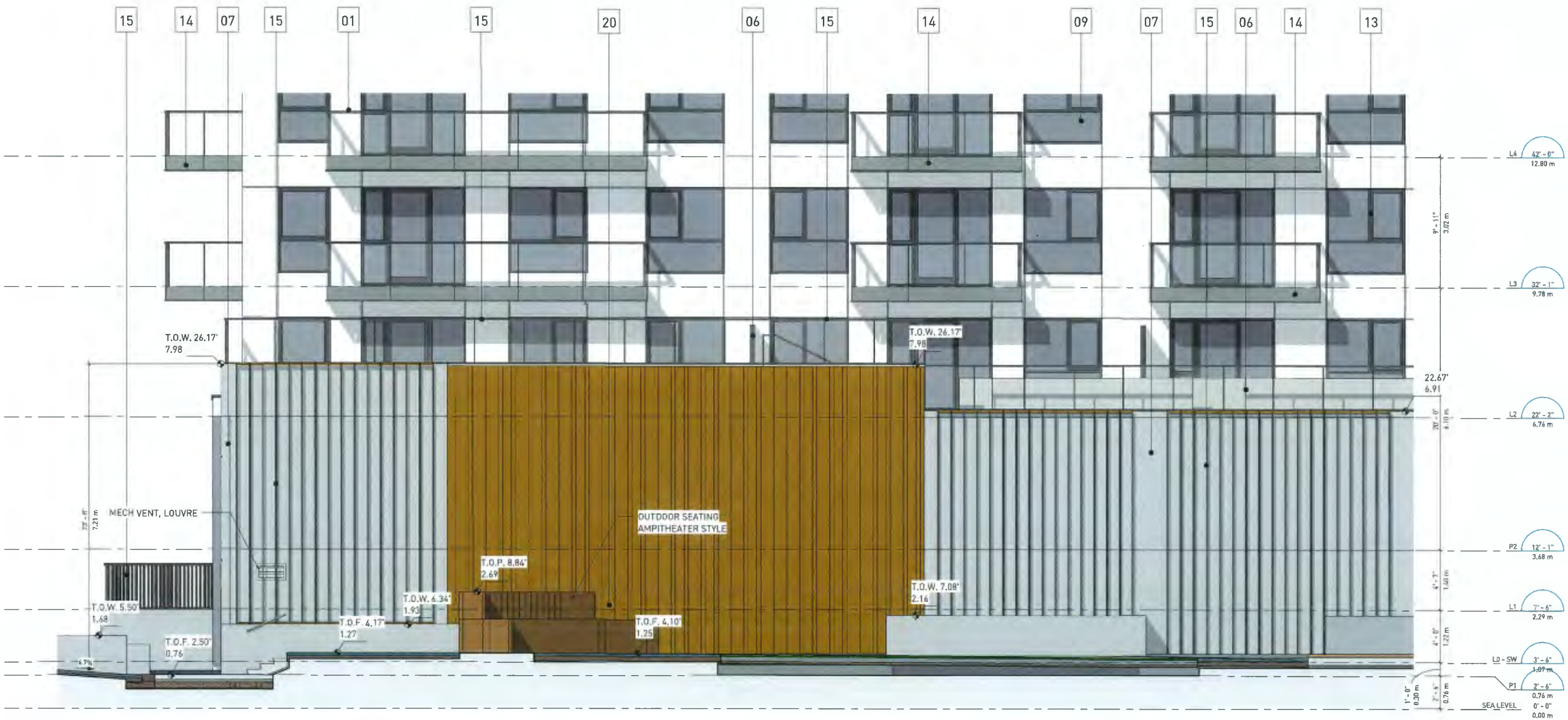
1 | ELEVATION - COURTYARD - NORTH WEST 1/4" = 1'-0"
