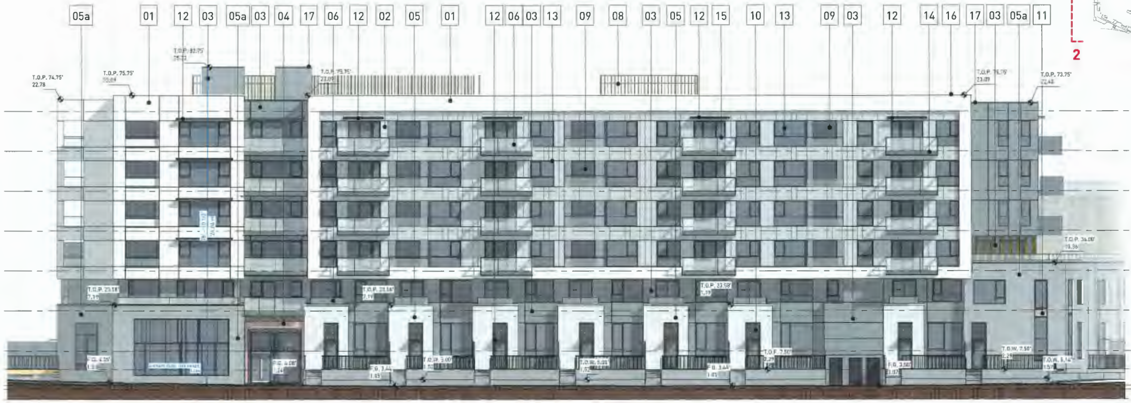
1 DP - BUILDING ELEVATION - SOUTH 3/32" = 1'-0"
