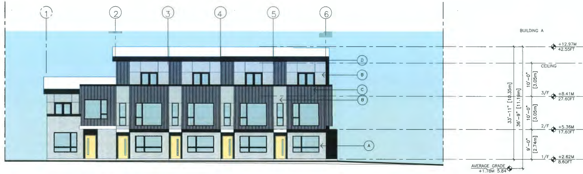
1 SITE ELEVATION WEST (FACING NO. 1 ROAD) A8 1/8" TO 1'0"
