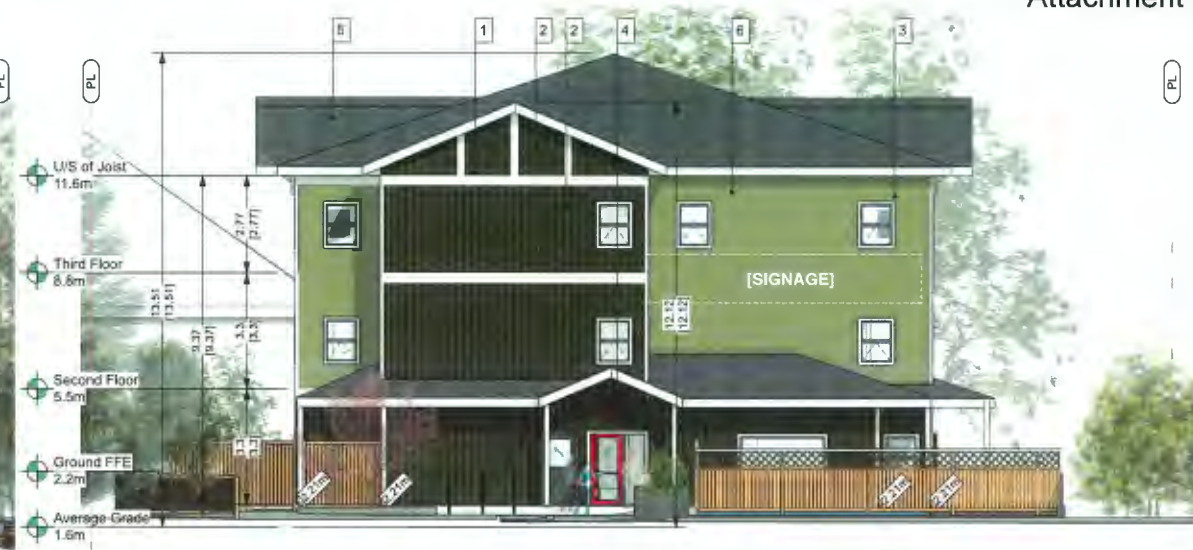
South Elevation 5-5 Scale: 1:96 [STEVESTON HWY]
