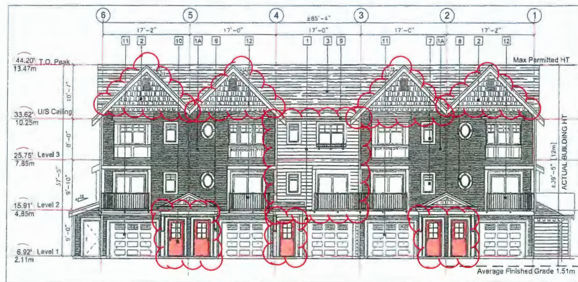
BUILDING 1 ELEVATION - NORTH Scale: 1/8"=1'-0"
