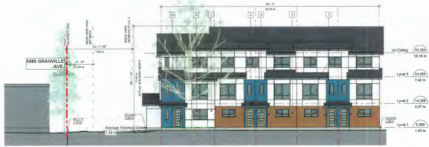
NORTH ELEVATION (ALONG GRANVILLE AVE.) - BUILDING 1 1/8" = 1'-0"
