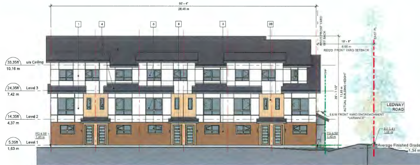
NORTH ELEVATION (ALONG GRANVILLE AVE.) - BUILDING 2 1/8" = 1'-0"
