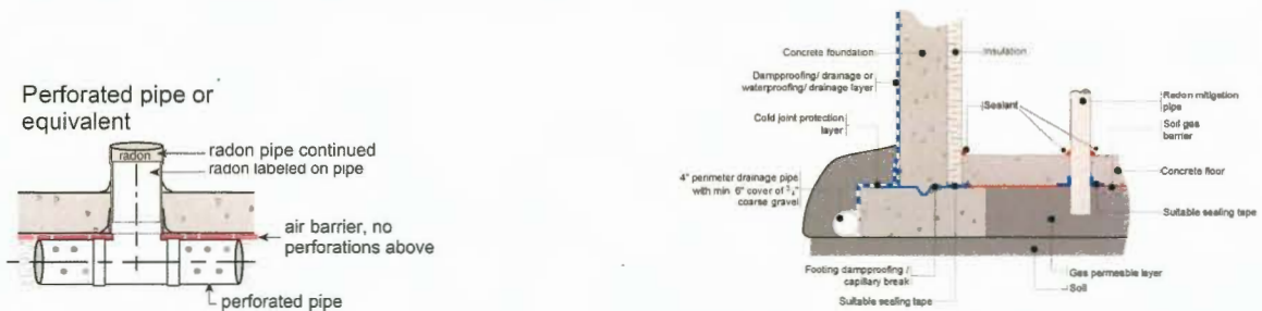
Figure 7.1.4.5.7 — Sealing sub-slab membrane horizontally to concrete footing when insulation is between the foundation wall and floor slab
