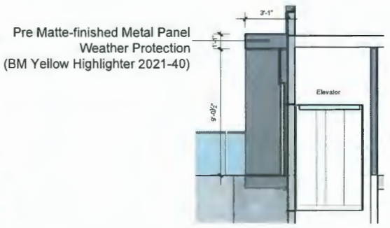
Elevator Weather Protection 6 Section Scale: 1:50
