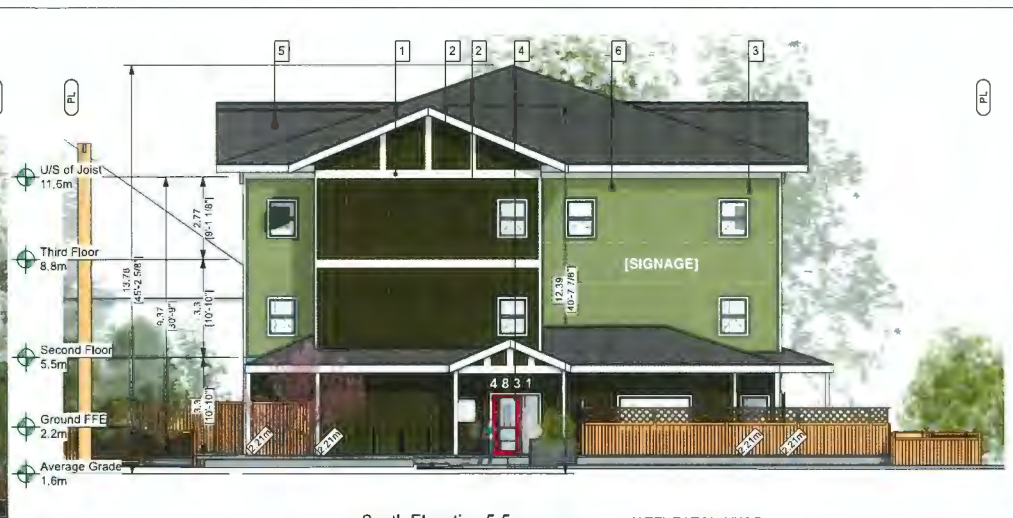
South Elevation 5-5 Scale: 1:96 [STEVESTON HWY]
