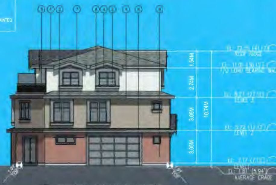
4 BUILDING A WEST ELEVATION SCALE 1/8"=1'-0"
