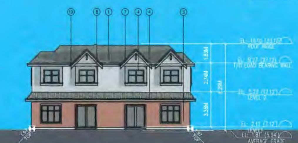
2 BUILDING D NORTH ELEVATION SCALE 1/8"=1'-0"
