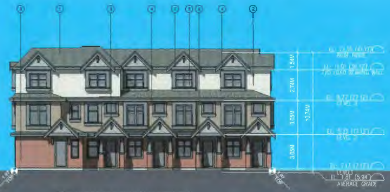
1 BUILDING A SOUTH ELEVATION SCALE 1/8"=1'-0"
