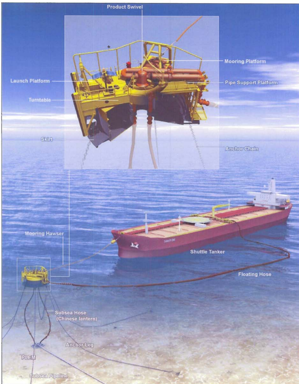
Figure 1 Typical Single Point Mooring Buoy Installation
