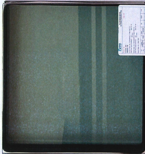
Solar Control Low-E Triple Insulated Glazing Unit Solarban 60®9mm + Air 12.7mm + Clear 6mm + Solarban 60®6mm
