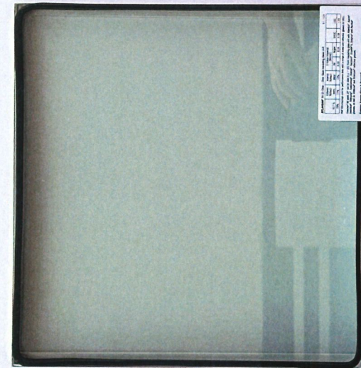
Solar Control Low-E Double Insulated Glazing - Door & Operable Window Solarban 60®9mm + Air 12.7mm + Clear 6mm
