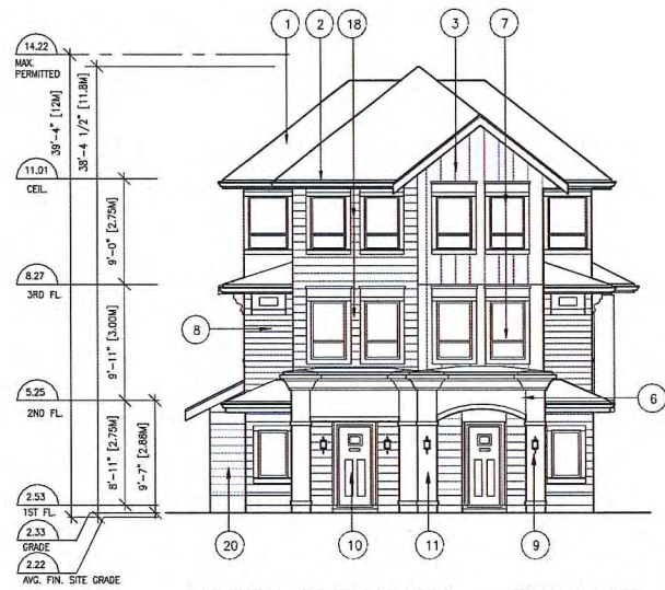
NORTH ELEVATION - BUILDING 1 SCALE: 1/8"=1'-0"
