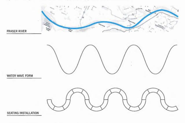
Figure 2 – Development of the seating form installation design.
