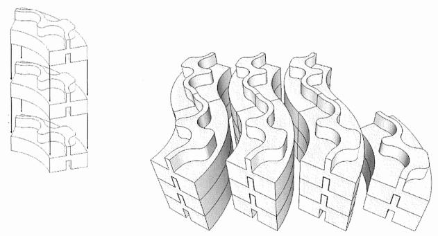
Figure 4 - All of the proposed benches are identical for ease of fabrication, and are easily stackable for compact storage.
