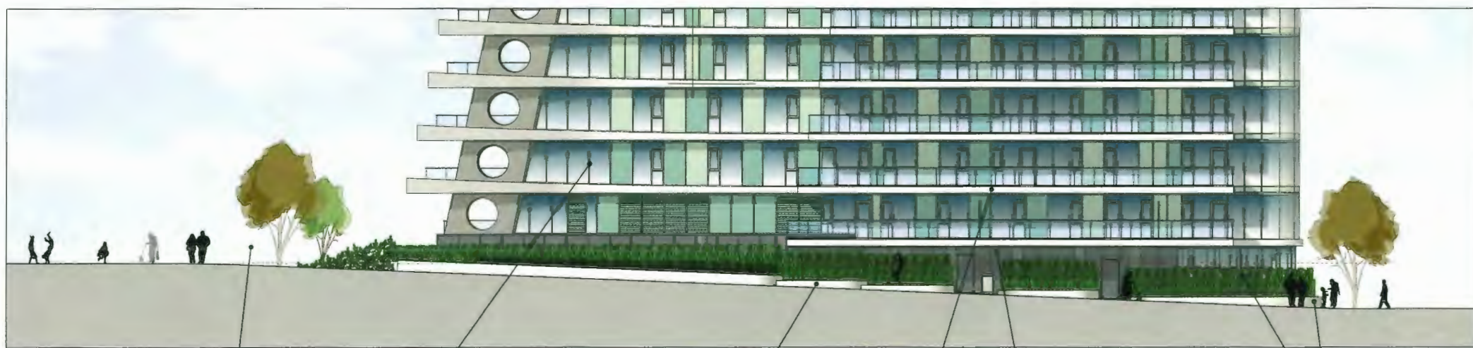
Lot C South Elevation • Capstan Way Dyke walkway and planting | Glazed window wall | Planter boxes with integrated benches | Private balconies | Fiber cement panel wall | Planter at south east corner | Curtain wall with translucent coloured glass
