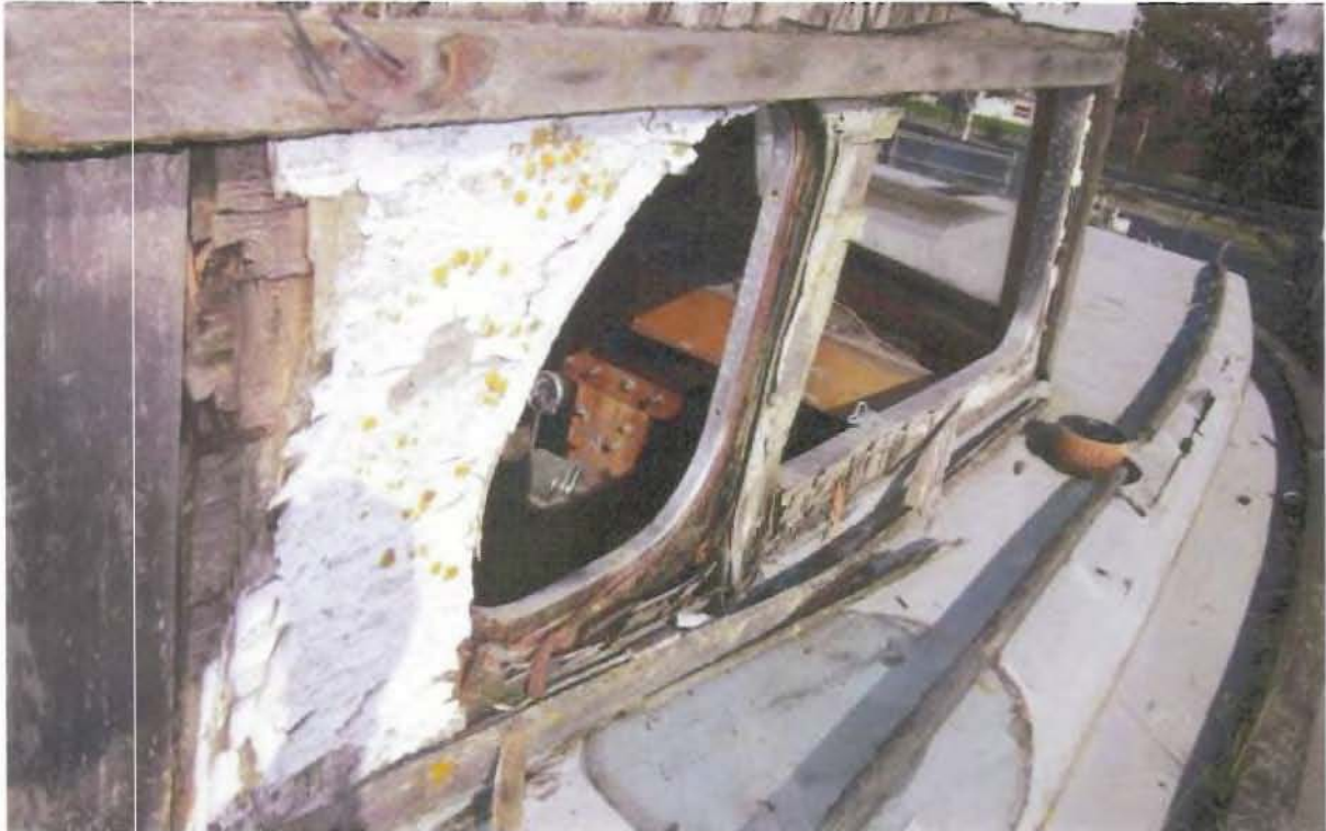
Photo # 3 Heavily deteriorated superstructure
