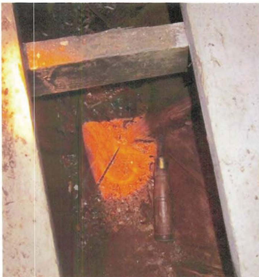
Photo #6 Detail of rib pulled away from hull
