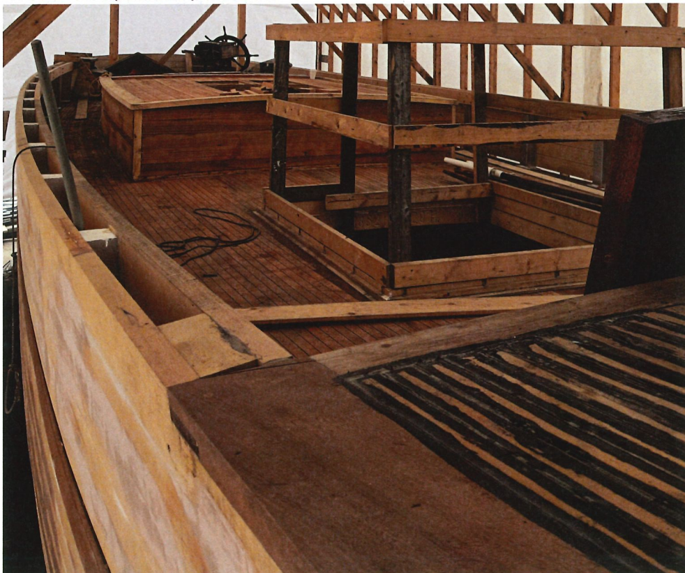
Hull frame complete sans pilot house.
