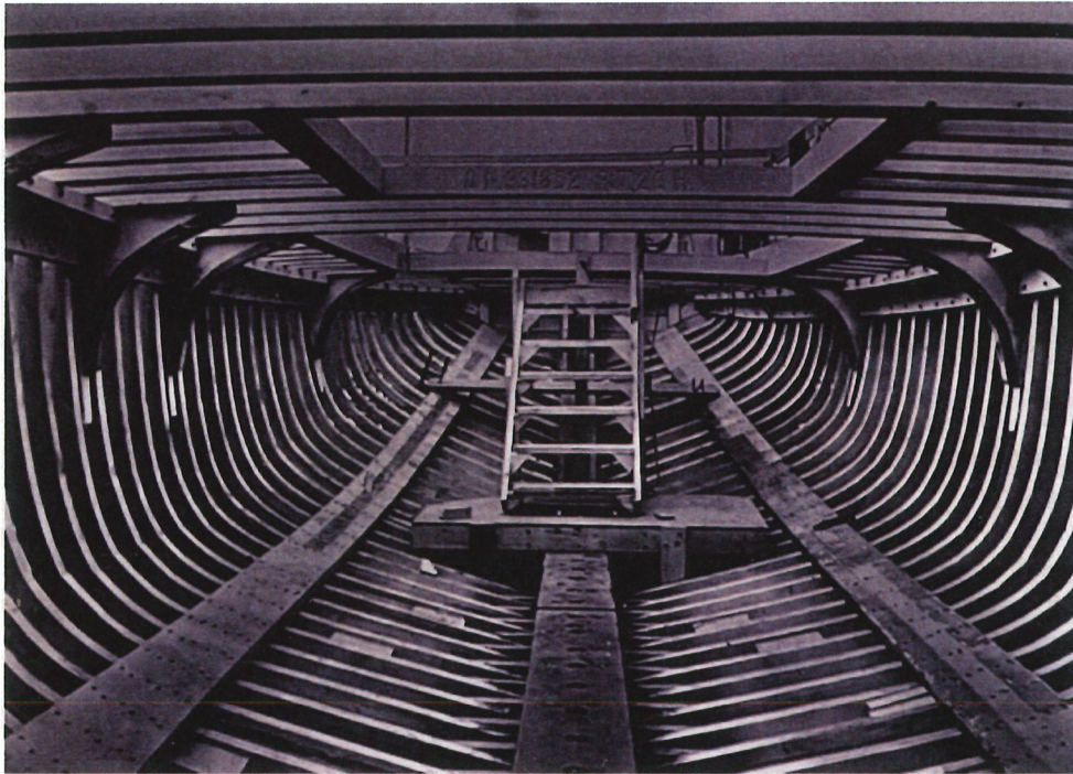
Hull frame complete sans pilot house.
