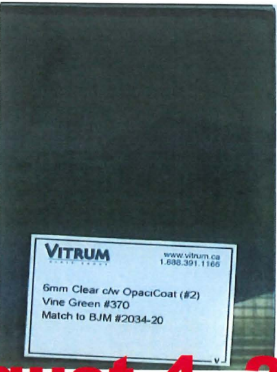
RESID'L TOWER SPANDREL PANEL COLOUR 2 BM-2034-20
