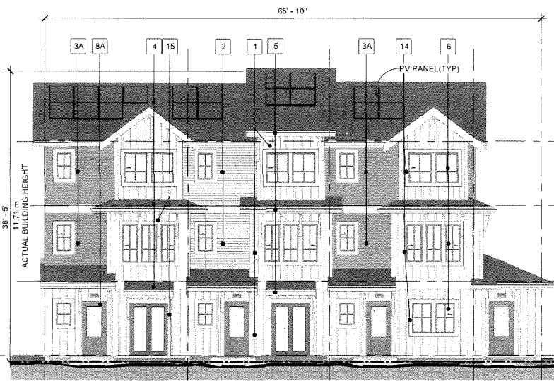
SOUTH ELEVATION - BUILDING 9 1/8" = 1'-0"
