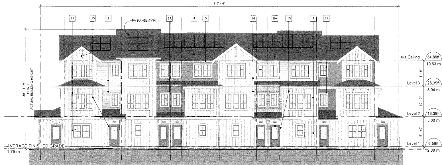
SOUTH ELEVATION - BUILDING 1 1/8" = 1'-0"
