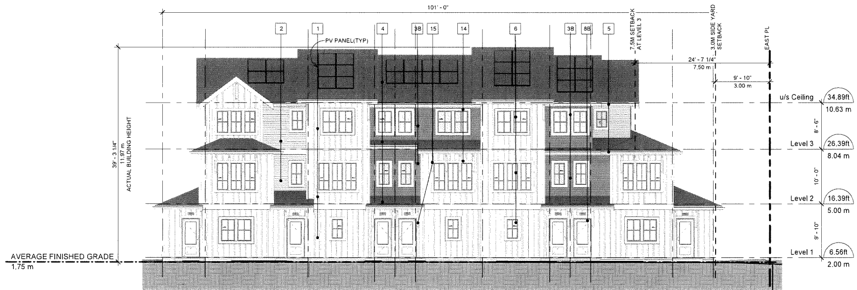
SOUTH ELEVATION - BUILDING 2 1/8" = 1'-0"
