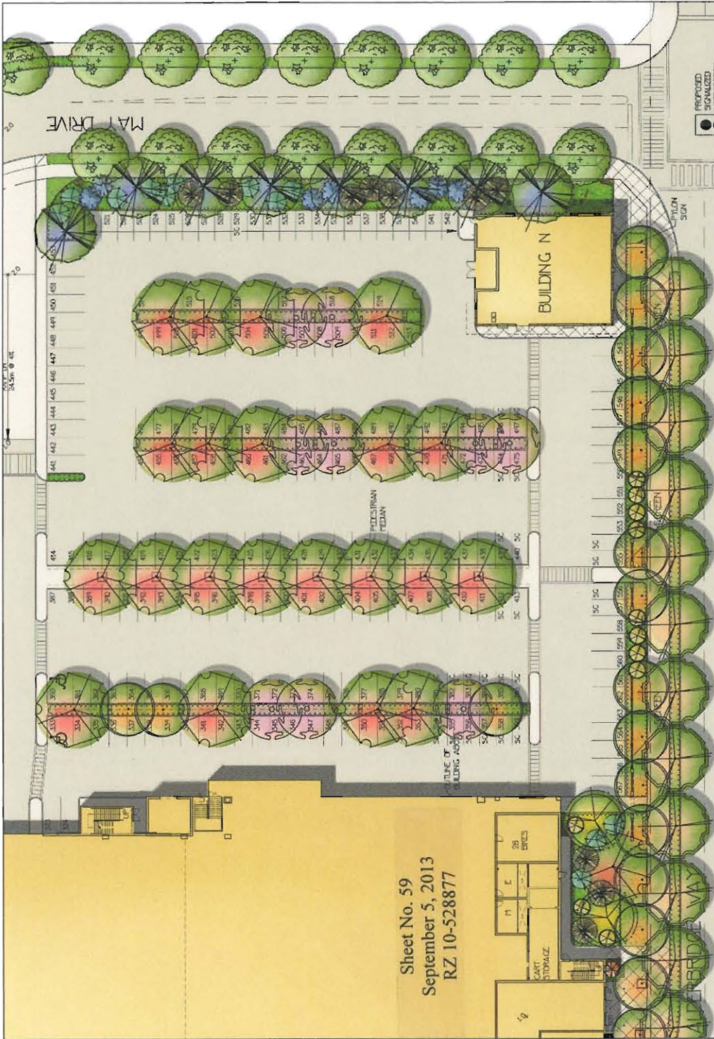
BIOSWALES TO MITIGATE STORMWATER
