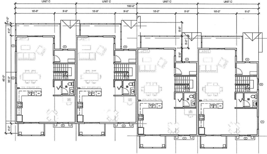
2 BUILDING 3 MAIN FLOOR PLAN 1/8"=1'-0"
