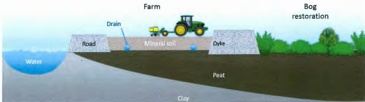
Figure 5. Cross-section of farm and bog restoration portions of the Garden City Lands, showing a 60 cm layer of mineral soil above native peat. Agricultural drainage will not penetrate the underlying peat, allowing it to remain saturated and acidic to prevent greenhouse gas emissions associated with drainage, fertilization, liming, and cultivation, all of which contribute to peat degradation. Mineral soil above the peat will be managed to increase organic matter content and sequester carbon.
